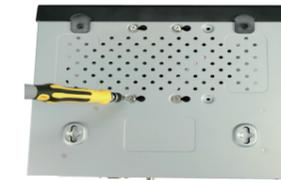
**Step 5:** Cover the top cover and fix it with screws.
